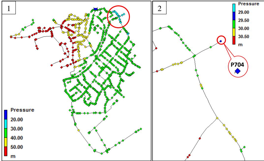
Figure 4.35. The location of the CP related to the least predicted pressure in the PSA (assuming -25% decrease of non-leakage flow) during winter season. CP (P704), on 15.01.2016 at 12:00 AM; min. pressure = 29.60 m, \Sigma Q_{(75\% \times \text{non-leakage}) + (\text{leakage})} = 69.46 \text{ m}^3/\text{h} and pressure upstream PRV = 32.05 m
