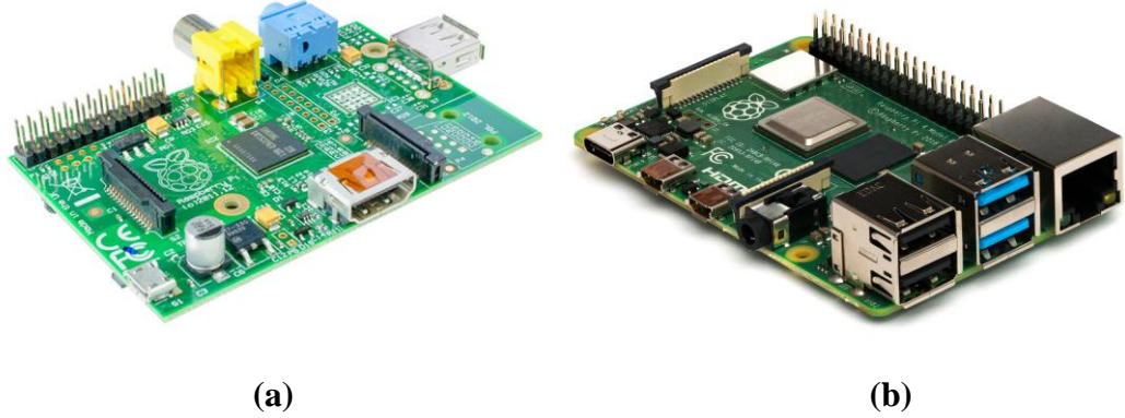
Şekil 1.4. a) Raspberry Pi 1 modeli (Sparkfun 2014); b) Raspberry Pi 4 modeli (Raspberry Pi Foundation 2019)
